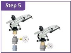
Connect the Raingun to the male thread of adapter and install the pressure gauge to the port given in the adapter
