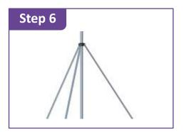
Spread the three Angular Support from the central riser at equal distance and place them on the ground
