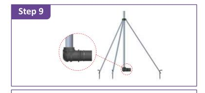
Connect the QFC (Quick Fit Connector) to the bottom thread of central riser
