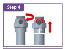
To dismantle the Raingun Adapter from the riser stand, turn it to 45 degrees anti-clockwise to unlock and pull it upwards
